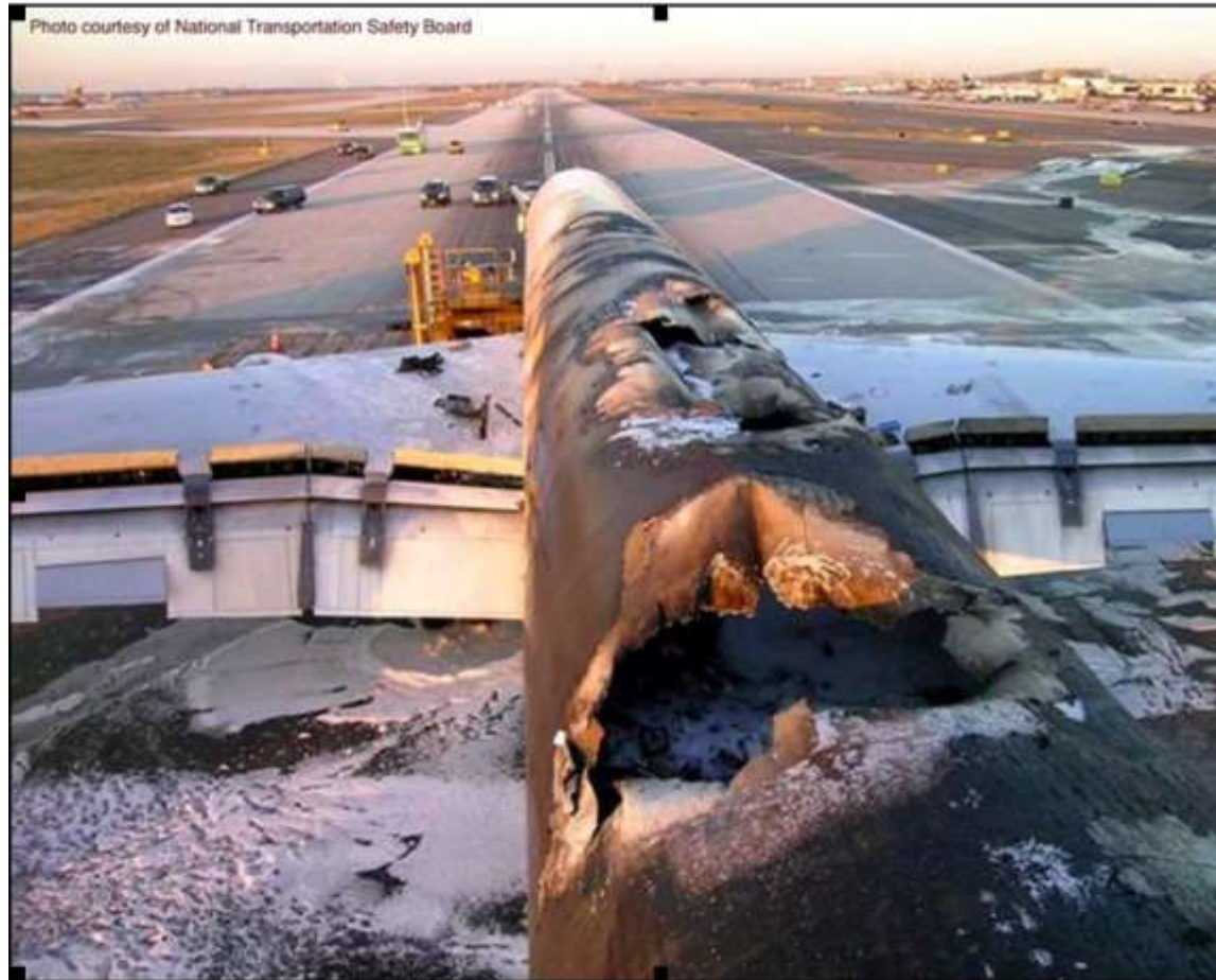
UPS Plane destroyed by lithium ion battery fire
