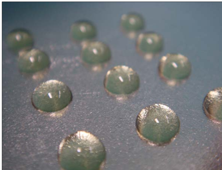
Figure 1. Non-stick, wear-resistant coating on stainless steel. The form of the droplets is an indication of the high contact angle.
